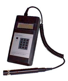
The instrument is capable of measuring entanglement points on textured and flat yarn at speeds up to 5000 M/min. Different amplification levels can be selected to suit various signal levels generated by a wide range of yarns and entanglement points. This makes the ETM3 suitable for all types of air jet application on draw texturing, draw twisting, draw winding, POY spinning and draw warping.
